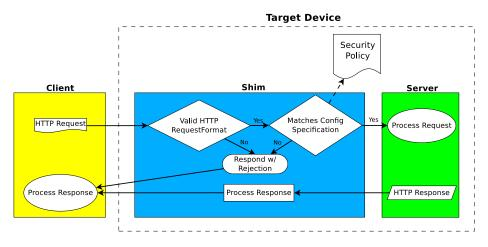
**Figure 1. Umbra Architecture**—A lightweight software "shim" runs on the embedded device and transparently proxies client requests, rejecting those that are malformed or that do not match a predefined security policy.
